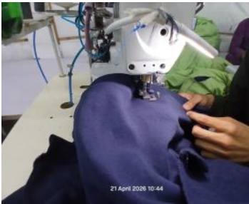
NC-Needle guard not installed.jpg
